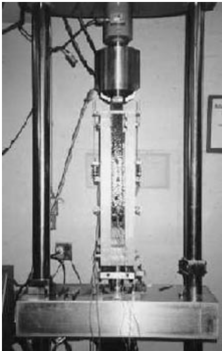
Fig. 2. Pull-off test experimental apparatus.
